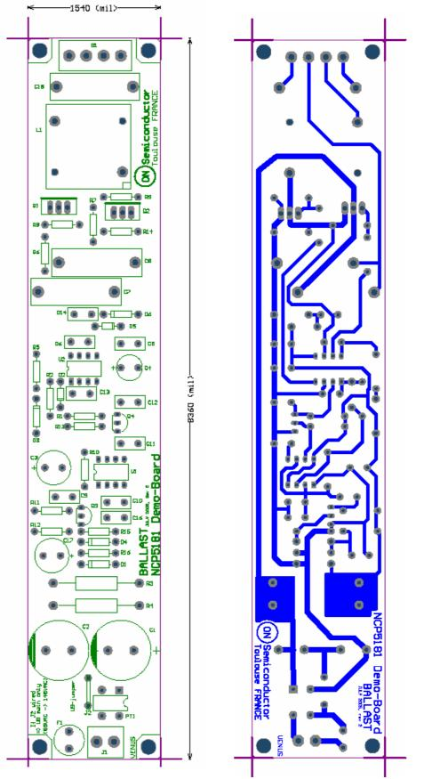
Figure 5. PCB Printout: Top and Bottom View
