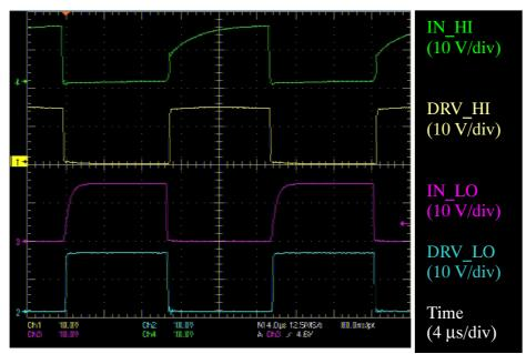
Figure 2. Input Output Timing Diagram
